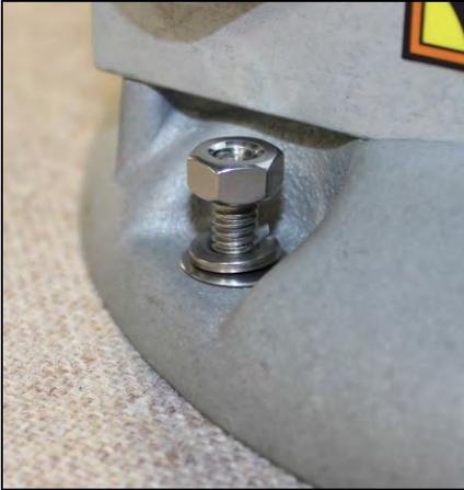
*Figure 15: Insert Nuts onto Hanger Bolts*
