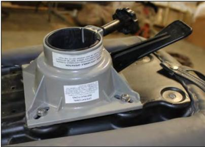
*Figure 4: Identify 2-7/8 Inch Spider Assembly*
