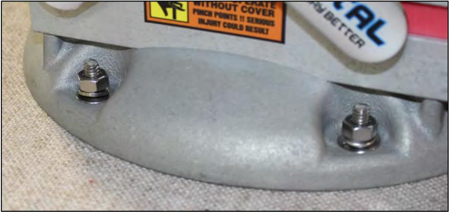
*Figure 17: Tighten Pedestal to Floor of Boat*
