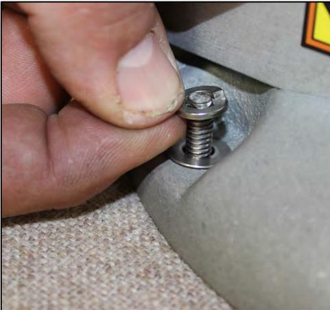
*Figure 14: Place Lock Washers over Hanger Bolts*
