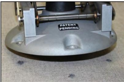
Figure 7: Align Hole Pattern with Holes in Floor
